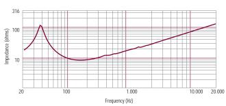
Impedance magnitude curve measured in free air.
