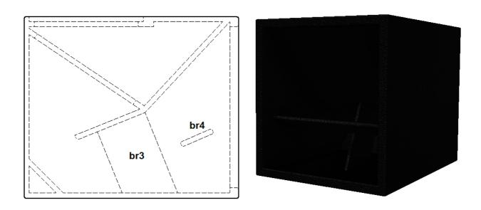
Bracing br3 can be made from a rectangle with the dimensions:  $303 \times 180$ ; where one corner is then cut off in a  $68^{\circ}$  angle. Bracing br4 can be made from a rectangle with the dimensions:  $564 \times 120$ .
