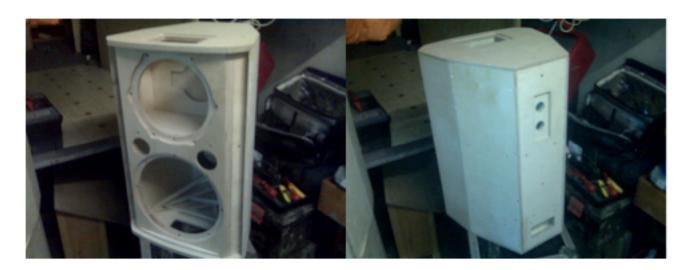
Designed in AutoCad, then precision cut out by CNC machine, out of the best 'BB' grade (void free) Baltic Birch Plywood.
